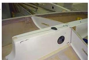
There is a large aluminum backing plate underneath the bow plate.
