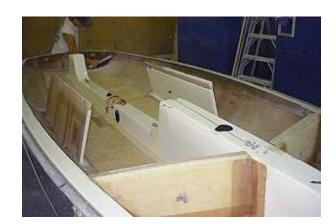
Note the reinforcements for the rudder gudgeons and the two blocks through which the shockcord runs that is attached to the board pull-down lines.
