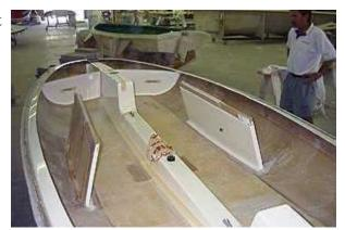
The mast step area of the strongback. Note the sidestay backing plate that has been glassed in underneath the edge of the hull.
