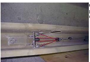
Center: Mainsheet block backing plate and 4:1 vang purchase (red line). Double block 'floats' on line going back up to deck. Single block is fixed.
