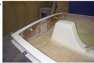
A look behind the bilgeboard box showing the reinforcements plus the aluminum plate for the board pivot bolt.
