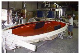
The MC mold consists of two halves that are bolted together prior to laying down the gelcoat. As you can see, the color is a dark red so that any blemishes on the mold can be more readily identified and corrected prior to starting the building process.
