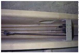
The MC strongback is fabricated in its own mold and all lines are installed before the strongback is epoxied into the hull. The next few pictures provide additional details in case you wonder how and where they attached lines and blocks.
