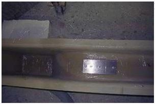
After the MC is removed from the mold, it is placed in a special cradle that properly supports the shell for the next steps in the process.
