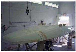
After the deck has been attached to the hull, it goes to the finishing area where blemishes are removed such as any center seam imperfections due to the clam shell mold. There is someone working under the hull!
